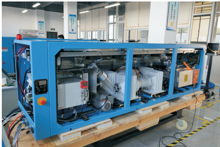
Wear-free 4500W轴快流CO 2 激光器
